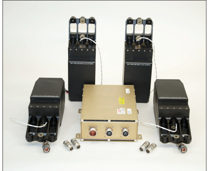
AVCS components with linear force generators for light helicopters
