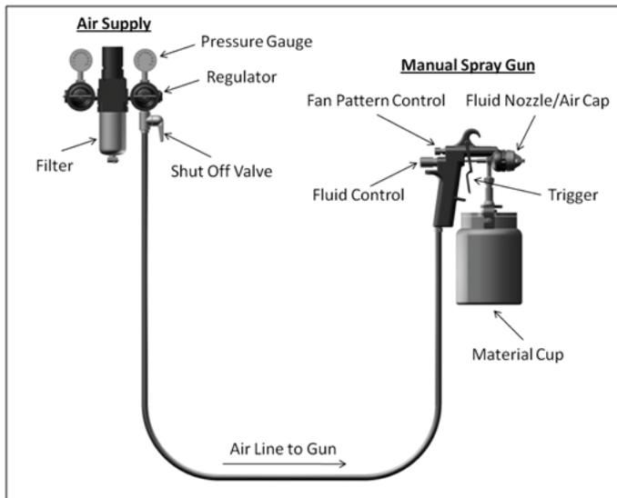
**Figure 9 – Manual Spray System with Pressure Pot**
