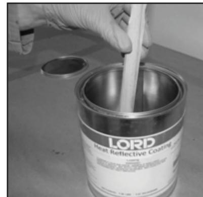
**Figure 4 – Mix with Mechanical Mixer**
