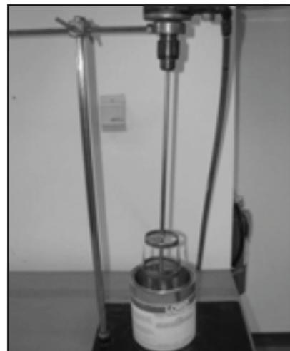
5. While mixing HRC A coating, add HRC B curative at 2.5% by weight and mix for 10-15 minutes (see Figure 5).
