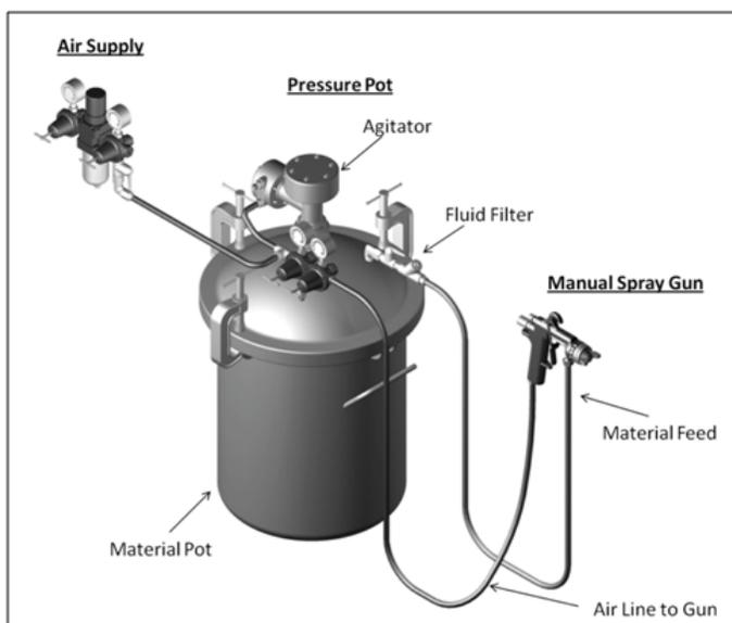
5. Set the atomization pressure between 1-3 bar (15-45 psi); adjust if needed.
